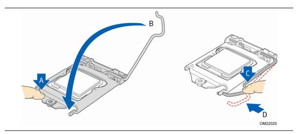
Figure 12. Secure the Load Plate in Place
